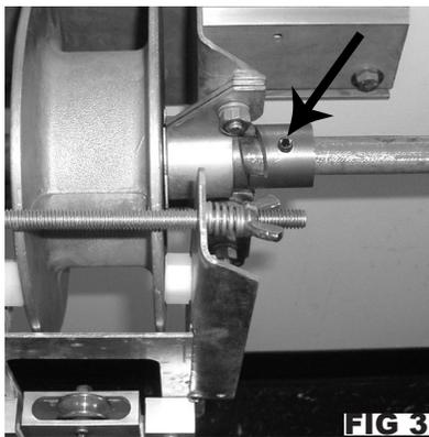
**FIG 3** - On the opposite end of the mechanism from your motor is a 4th pin that rarely breaks. (080123 SHEAR PIN 1/4 X 1 1/4)
