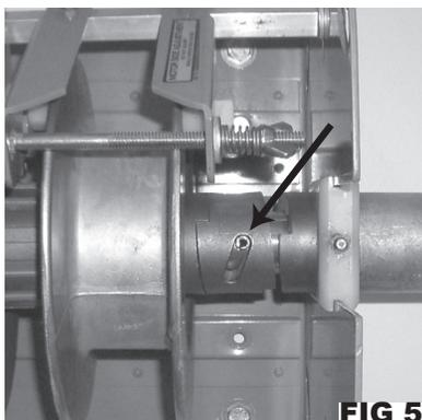
**FIG 5** - If you have a Model II system it looks like this and there is only one shear pin located on the farthest side of the rope reels from the motor. Follow the procedure above to replace the pin. (080101 SHEAR PIN 1/4 X 1- 1/2)
